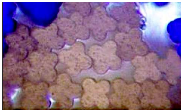
Figure 1. Cross-sectional view of X6300 nylon. Advanced spinning technology produces a four-channel cross-section for permanent moisture management performance.
